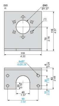
(1) 6 holes  $\emptyset$  7 for CHC M6 screws at  $60^{\circ}$  on 60 PCD
