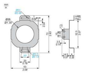
(1) 4 holes Ø 3.2. M3 x 6 screw fixings.
