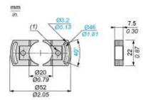
(1) 2 holes  $\emptyset$  4 at 180° on 30 PCD. TC M4 x 5 screw fixings
