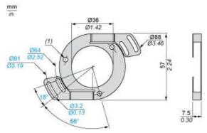
(1) 3 holes  $\varnothing$  4.1 at 120° on 48 PCD. TC M3 x 6 screw fixings
