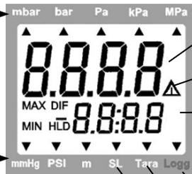
**Main display:** shows the measured value of CH1
