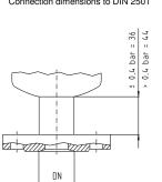
Miniature flange for vacuum systems DN 10 ... 32 Connection dimensions to DIN 28 403
