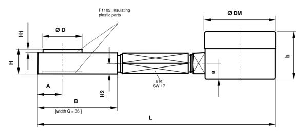
Remark: Couplings of the hydraulic force transducer must not be disconnected! In case of violation there will be no guarantee and no measuring function.
