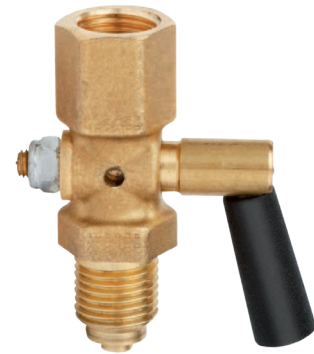
Stopcock Female / male G \frac{1}{2} / G \frac{1}{2} B, DIN 16261, PN 25
