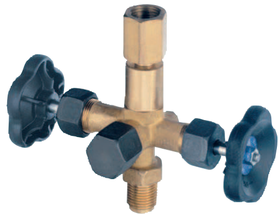
Shut-off valve with separately isolated test connection per DIN 16272, LH/RH union/male G ½, with test pivot M20 x 1.5, PN 400
