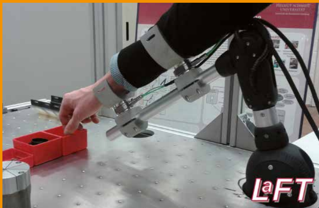
Manual workstation support system with human-machine interface for the production of the Manufacturing Technology Lab (LaFT) at Helmut-Schmidt University in Hamburg
